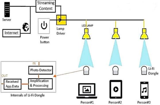
Fig. 1 The VLC transmitter and receiver.
