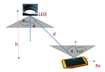
Fig. 2 Tx and Rx with a Lambertian emission.
