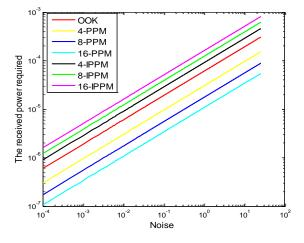
Figure 4 Received power required (W/m<sup>2</sup>) for OOK, LPPM, IL-PPM modulation schemes at  $R_b$ =1.6 kbps in the dark.
